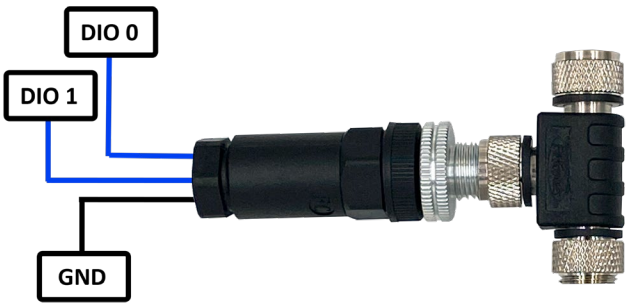
Figure 1: M12.8-T-SPLIT and M12.8-S-M-FM accessories for Discrete I/O access
